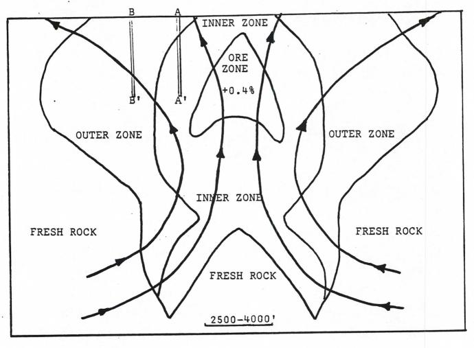
Fig. 3. FLUID CONVECTION and RESULTING ALTERATION ZONE
